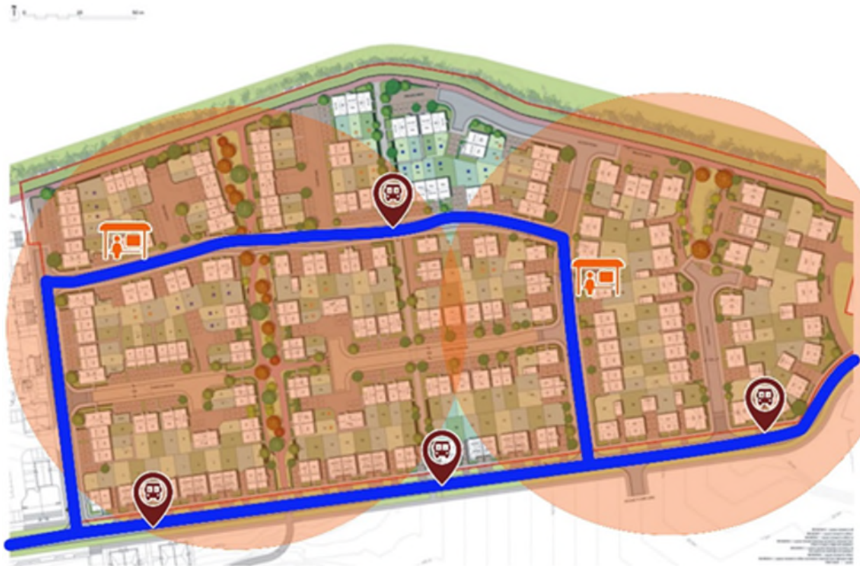
Figure 7 - Determined bus stop layout within a proposed new development but with the potential of bus shelters.
