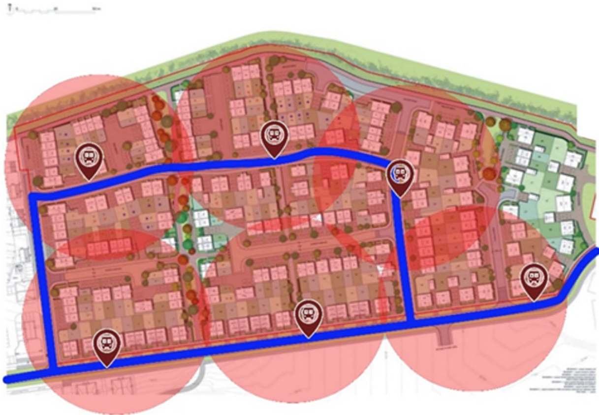
Figure 5 - Example of the 100m radius stop points and the locations of bus stops required.
