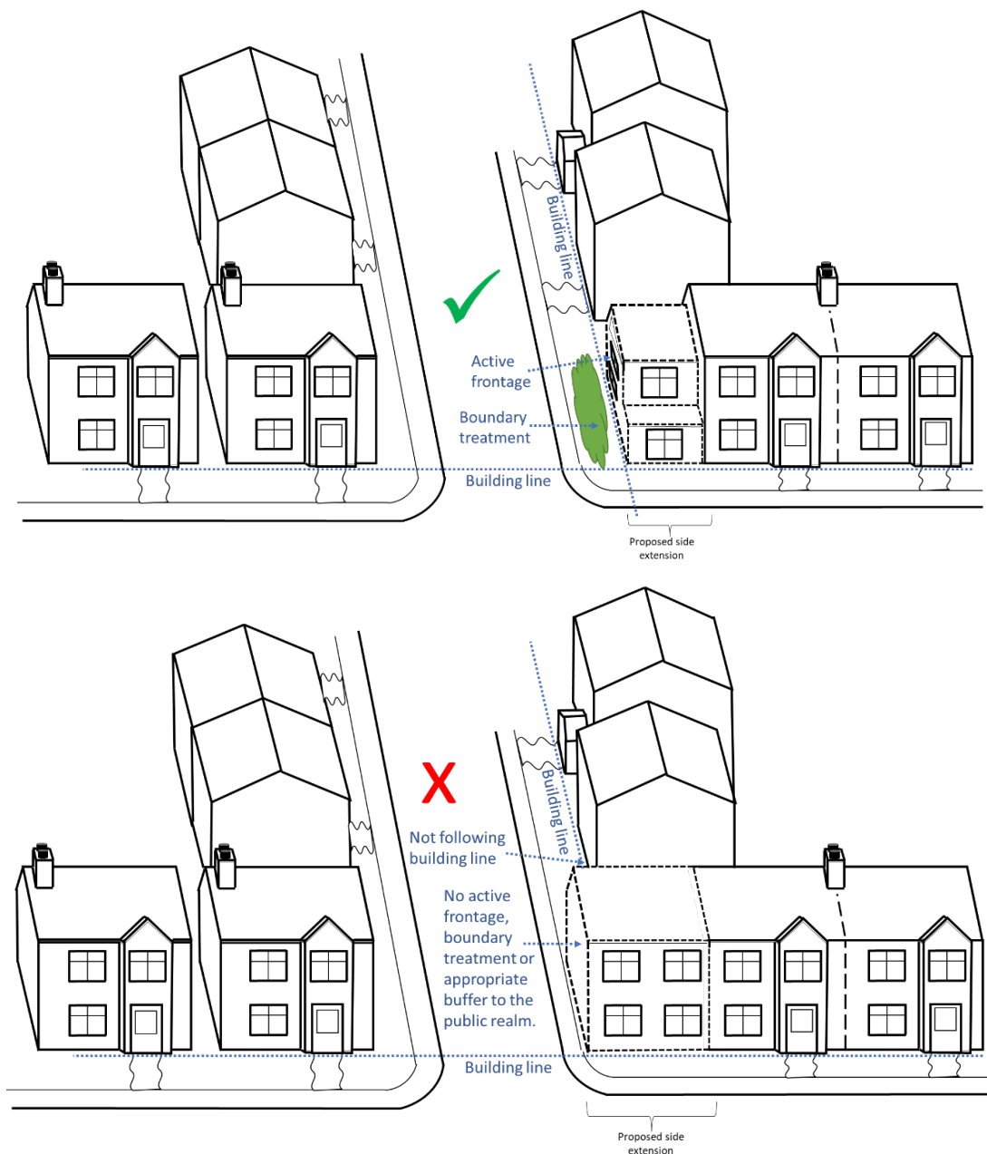
Figure 3.3: Side Extensions on a Corner Plot
