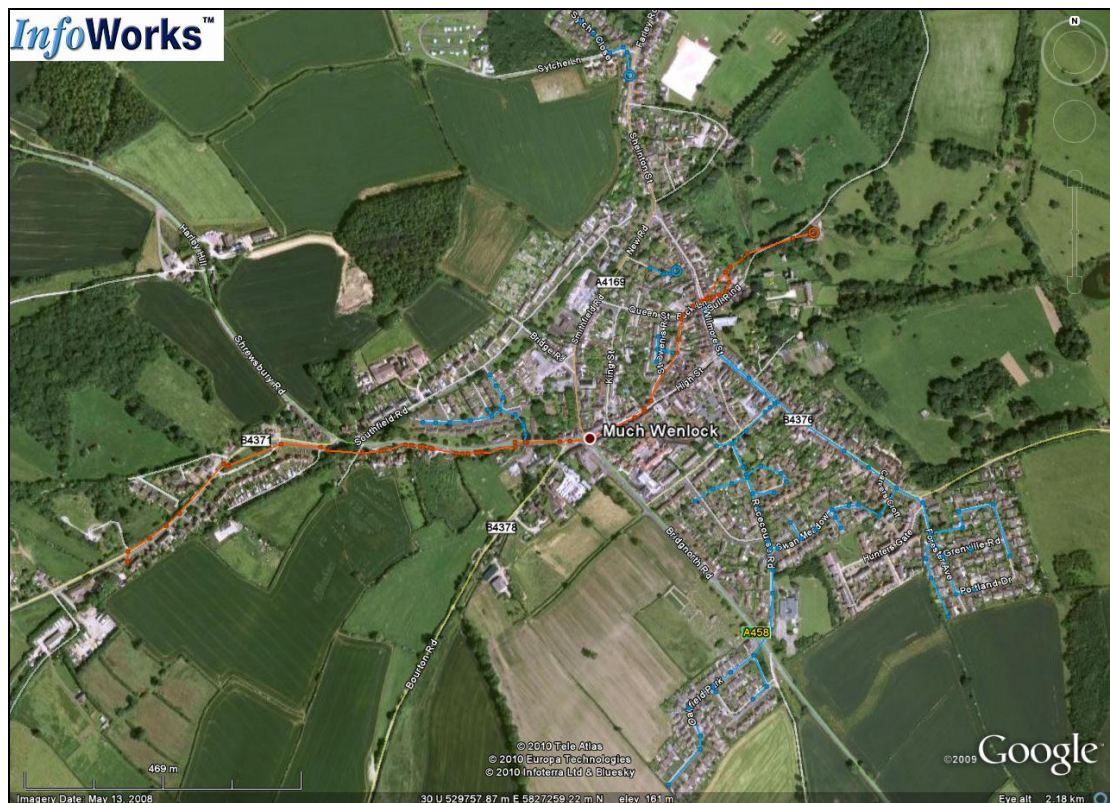
Figure 12 – InfoWorks integrated model extents developed by Mouchel: town culvert (red) and surface water sewers (blue). Google Pro licence 156330.
