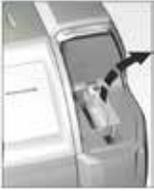
Remove the used Test Cartridge from the cartridge chamber and discard it in a suitable waste container. Insert a new Test Cartridge or close the lid manually.
