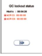
If the control level is specified it is required to run **two** passed controls, both control level C I and C II, to reset the QC lockout interval and unlock the assay for patient testing.
