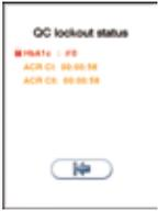
If no control level is specified, it is required to run **one** passed control, control level C I or C II, to reset the QC lockout interval and unlock the assay for patient testing.
