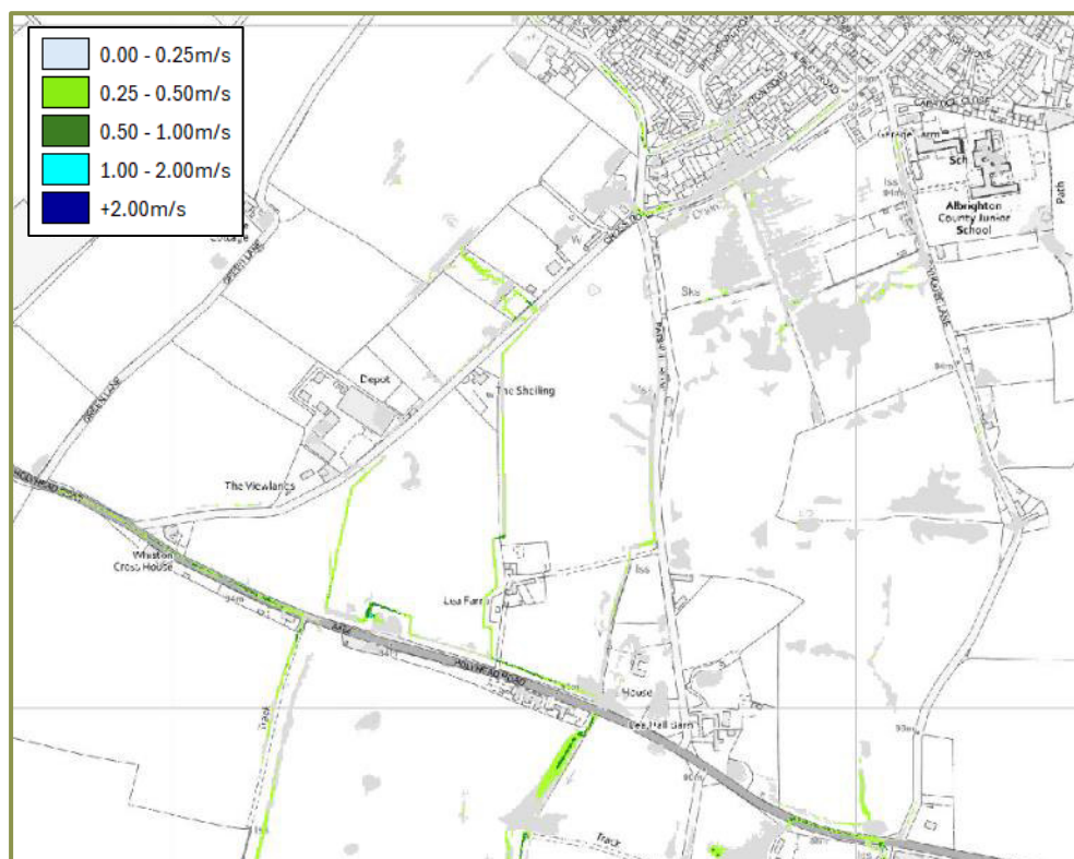
Figure 5.8: Flood Velocity Mapping – 1000-year (Run 017)
