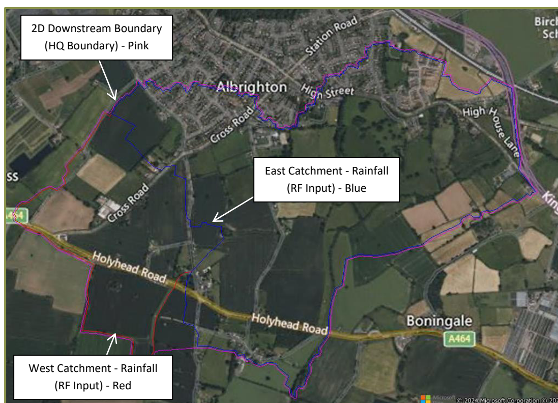
Figure 2.10: Peak Flow Calculation and Input Locations
