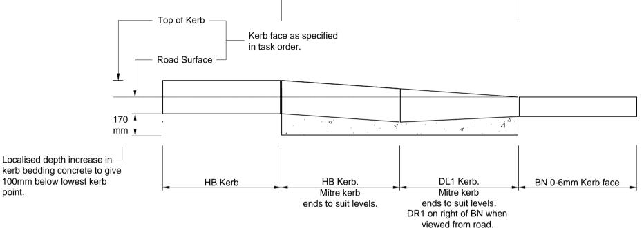
Or use similar manufactured precast concrete double dropper kerb products, although these units too would require mitre cutting to give a 0 to 6mm BN kerb face.
