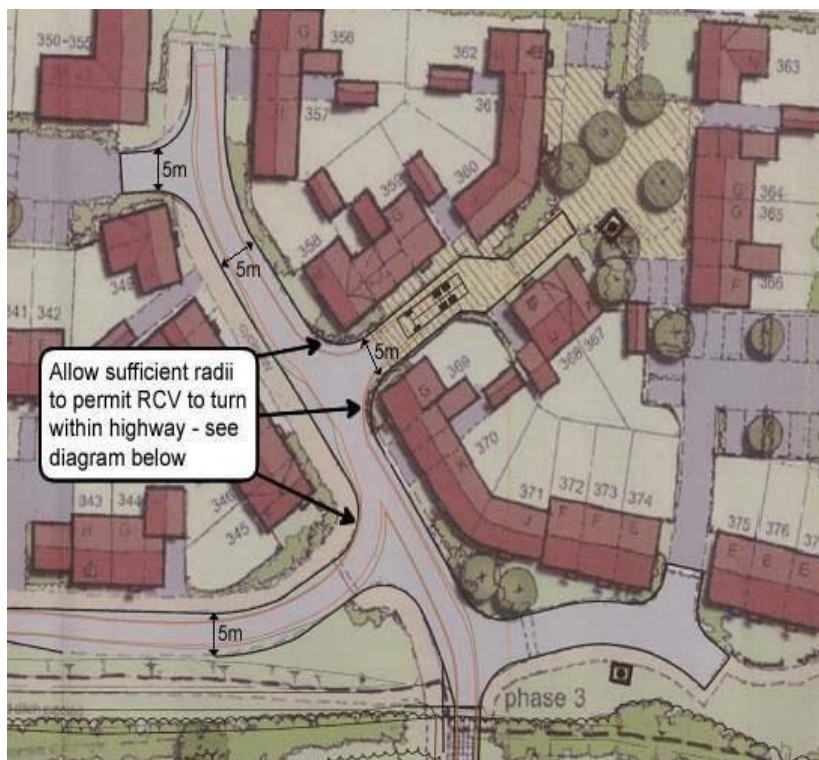
Example vehicle tracking plan. Orange lines indicate vehicle route
